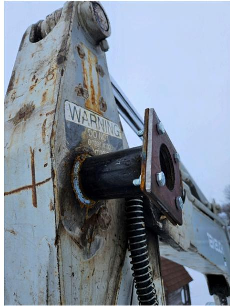
**Angle Tube #1 to allow for the GPS mount pivot point to be positioned above the boom-end pivot point, avoiding obstruction from the flange removal bolts when Tube #2 is inserted.**
