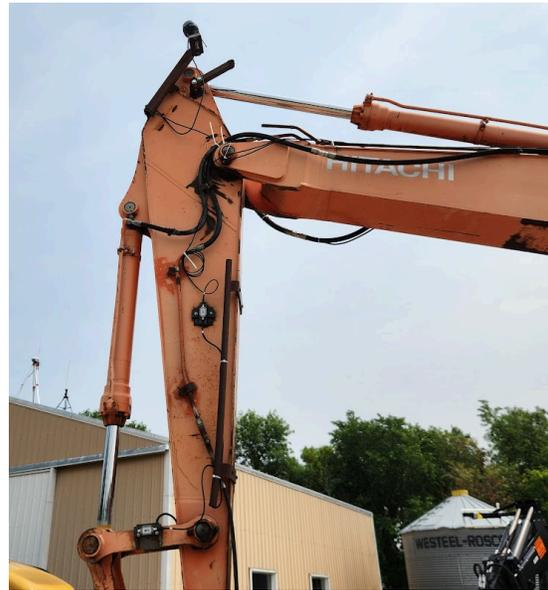
**Route the GPS cable through the loop on the GPS mount,** connecting it to the main harness. Secure any excess cable, ensuring sufficient slack for full GPS mount movement.
