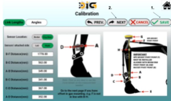
4. For precise elevation calculations, input the offset distance and direction if the GPS mount is not vertically aligned with points H and B. If it is aligned, maintain the 'Aligned' setting and proceed.
