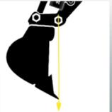
4. Now, slowly move the stick until the link connecting the A-B pivots is vertical. Use a plumb bob if necessary to ensure both points are aligned vertically. Once this is achieved, click the "Yes" button below.
