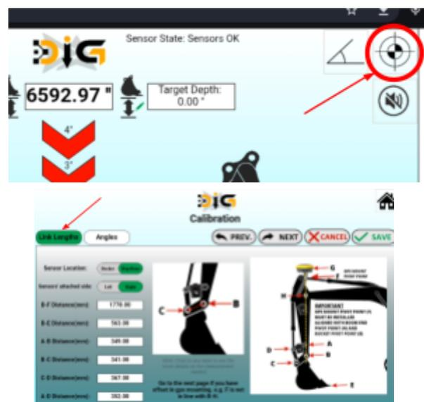
2. All measurements should be taken from the center of each link. Measure twice for best results, and convert measurements to mm (1cm = 10mm).
