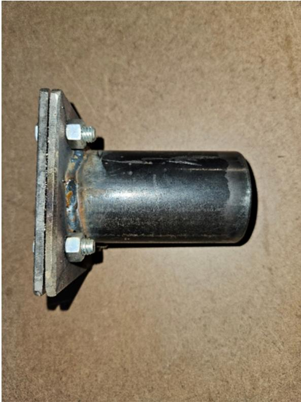
**Tube #1:** 2" ID SCH80 with GPS mount and counterbalance removal flange attached
