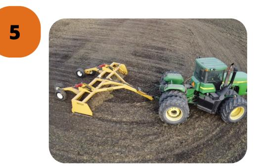
Begin working. Ditch Assist will calculate the design elevation at your location and set this as the target
