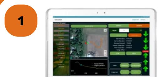
To create a flat, level area, lower the implement blade to the desired elevation, enter a **Target Grade** of **0**, and start working
