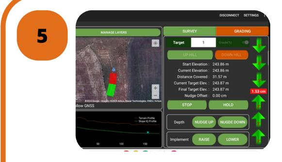
Monitor plow height on design profile during run. At end of run, hit STOP and manually raise plow
