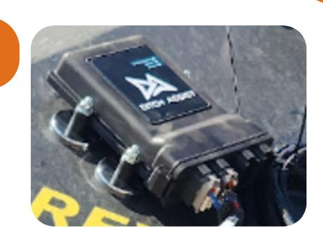
Install Control Module on implement using magnet mounts, ensuring line of sight to cab
