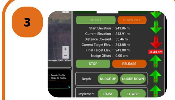
Always install UPHILL. Hit START then HOLD to lower plow into start hole to indicated depth
