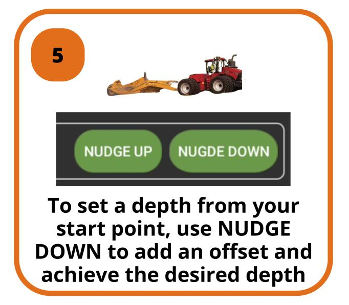
This method will maintain a constant grade calculated in a straight line from your start location to your current location. To implement a grade break, hit STOP > RESET and then enter a new grade and continue from that point.
