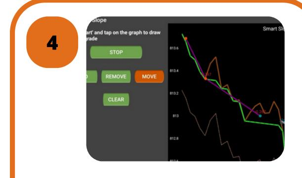
Move or remove a vertex point by first tapping it so it changes color then using appropriate buttons
