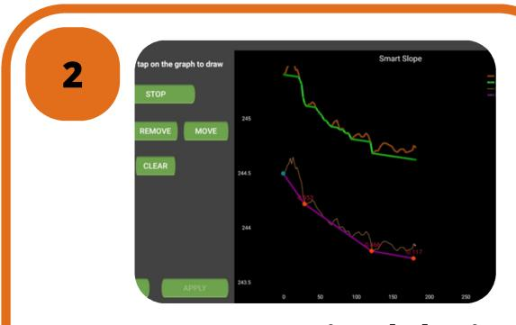
Create a Customized design observing minimum depth and grades as well as maximum depths
