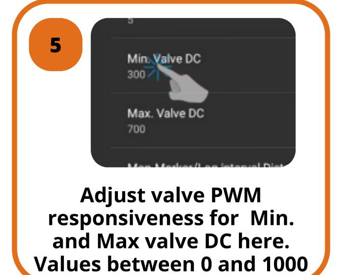
For larger implements with higher flow requirements you may need to increase the Min. and Max. DC values for faster response movement. Smaller implements may require lower settings to prevent jerky movement and overshooting the target.
