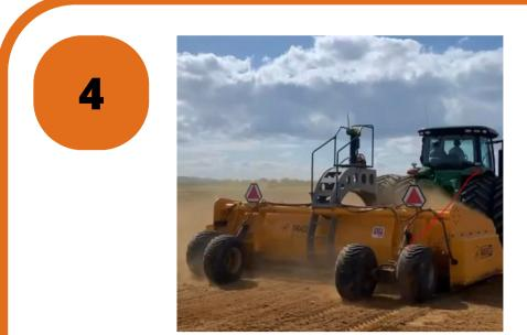
Ditch Assist will automatically expand the original survey line, stretching it out at 90-degree angles on both sides
