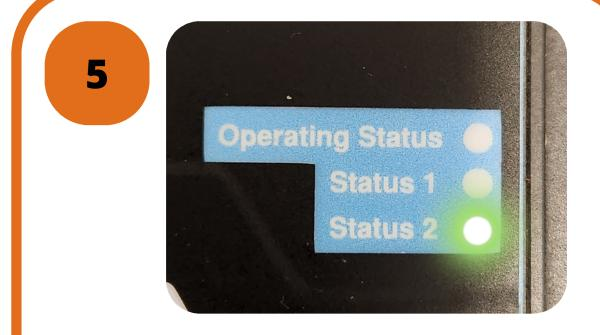
On the Ditch Assist Control Module, the **Status 2** light will blink if NMEA messages are received
