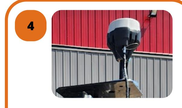
Connect GPS to Ditch Assist and power on. Ensure GPS is outside and has clear sky view for messages to send
