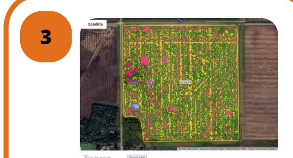
Easiest way is to use the free Image Georeferencer on the Ditch Assist website to generate the .jgw file
