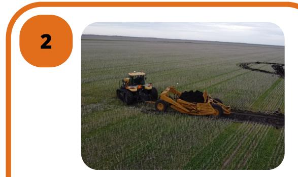
The implement should move to the target elevation. Begin driving the original survey route
